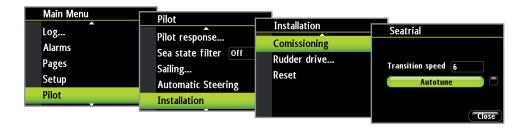
The automatic tuning process is also verifying/adjusting the Rudder zero alignment made in Dockside setup. Automatic tuning is a procedure that is not required for the Pilot to function as it is preset with steering parameters that should steer most boats in the 30 - 50 foot range.
