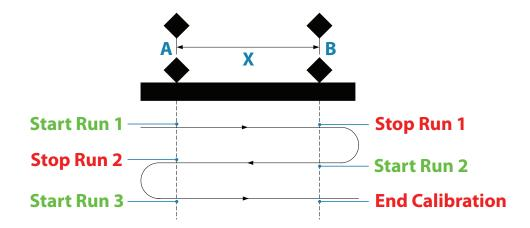
As the boat passes marks A and B on each run, instruct the system to start (Start Run) and stop (Stop Run) and finally OK to end calibration (End Cal Runs).
