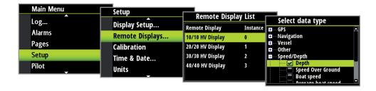
→ **Note:** You can differentiate between displays in the Remote display list by setting an instance number when you configure the remote display.
