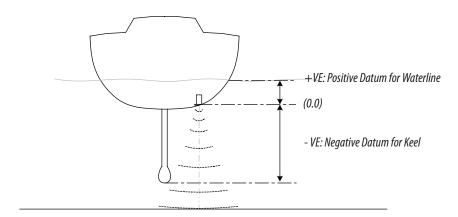
Setting the depth offset displays depth readings from directly below the keel or propellers of the boat, or from the waterline to the seabed. This makes it easier to see the available depth, taking into account the draught of the boat.
