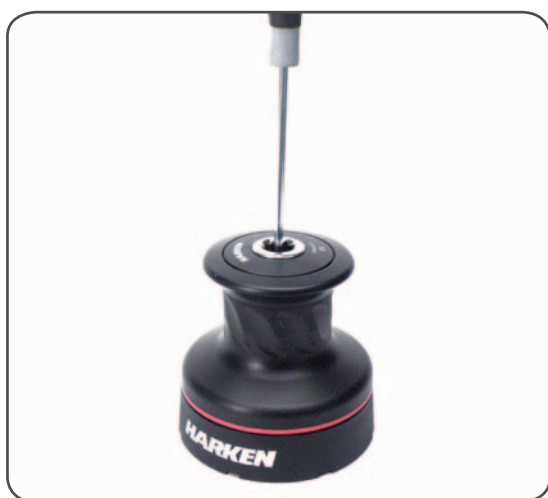
1. Unscrew the central screw ( \approx 2\text{Nm}/18\text{ in-lb} )
