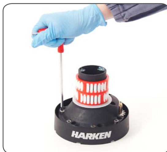
5. Remove the socket support n°21
