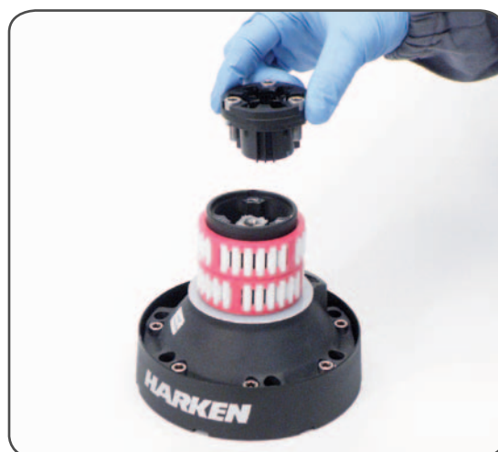
5. Remove the socket support n°21
