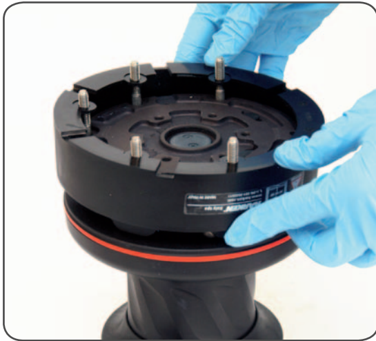
4. Reposition the skirt n°2 in its housing
