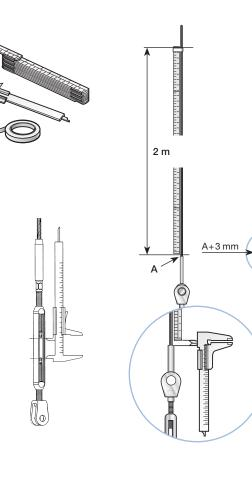
Hint! Count how many turns on the rigging screw corresponds to 1 mm elongation (5% of the breaking load). Make a note of it. This is useful to know if you ever need to tension "another 5%".
