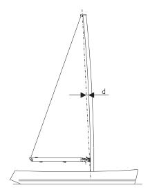
2. Tune the D1 shrouds until you have achieved the desired prebend of **100 mm** for the conventional mast and **40 mm** for the furling mast.
