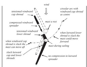
Some rigs are equipped with diamond shrouds (from the forestay attachment via the spreader tip to the mast heel). These diamonds are rigged to maintain compression in the leeward spreader. Consequently none of the diamonds must go slack.
